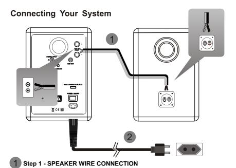
Connect the **RED** (+) and **BLACK** (-) terminals from the left speaker to the corresponding terminals on the right speaker using the included speaker wire. Be sure to match the red-colored side of the speaker wire with the **RED** (+) terminals and the black-colored side to the **BLACK** (-) terminals on each speaker.
